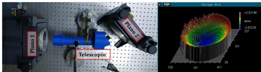
Figure 3: The wavefront error is equivalent to 0.55\lambda . It is within an allowable error close to 0.5\lambda error according to Walker B. [4, p.23]. As can be seen, the total wavefront error indicated by the software is 1.1\lambda ; but, since the wavefront travels through the telescope twice, the wavefront error is half that.
