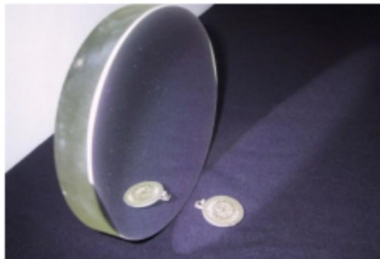
Photo 1: Aluminum and Magnesium fluoride coated first-surface mirror.
