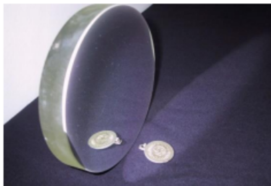
Figure 1: Aluminum and Magnesium fluoride coated first-surface mirror.
